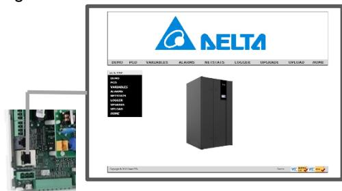
**Ready networks** connection and built-in WEB server function makes you convenient to whether monitor or control via Ethernet network from anywhere you are. All parameter displays on the WEB is simultaneously reporting the same value with front display of the RoomCool unit.
