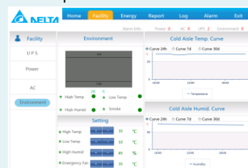
Critical component status: Hot & Cold isle
