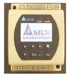
New generation smart relay, to cater to the increasing need in Industrial automation is also being developed. This fills a gap in the product portfolio of IABG and strengthens the market position of Delta in Industrial automation in India. The uniquely designed editors available on PC/Mobile and handheld design makes these devices extremely user friendly.
